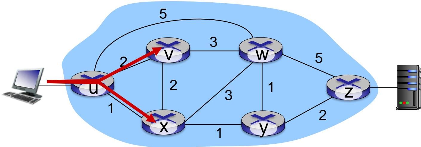
Q: what if network operator wants to split u-to-z traffic along uvwz *and* uxzy (load balancing)?
