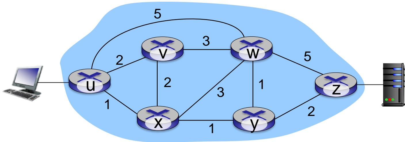
Q: what if network operator wants u-to-z traffic to flow along  $uvwz$ , x-to-z traffic to flow  $xwyz$ ?
