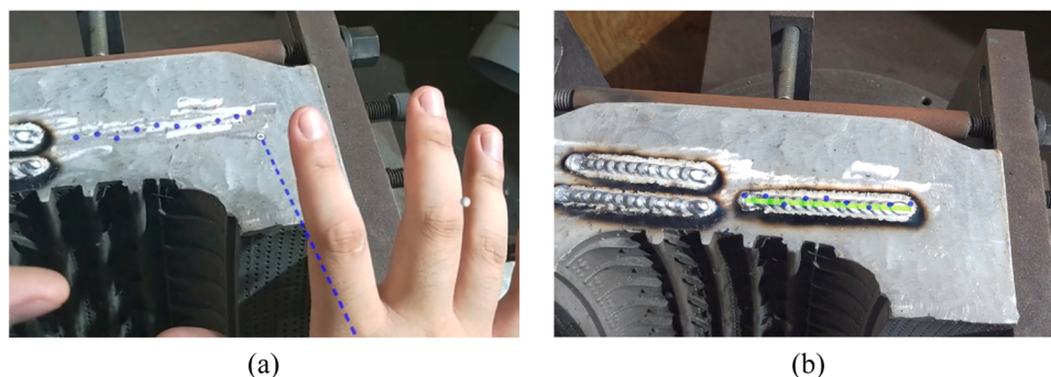
Fig. 19. Deviations of line tracing in the robotic welding process: (a) hand ray input and (b) the welding result on the tire mold.
