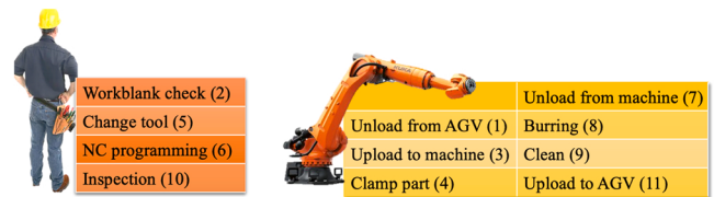
Fig. 14. Manufacturing system configuration of selected solution 2.
