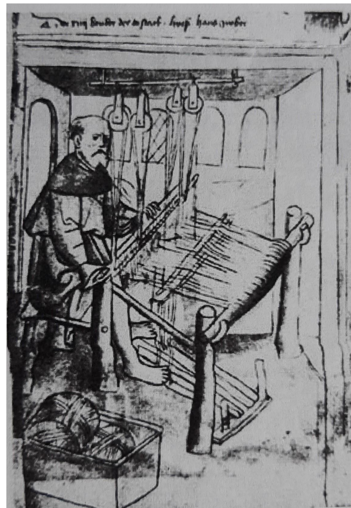
Weaver working at treadle loom with harnesses suspended from above. Late 14 th century, Germany. (Hann, 2005, 37)
